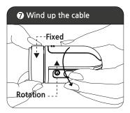
After using speaker, wind up the cable by holding the winder with one hand and turn the speaker body with the other. \*6)
