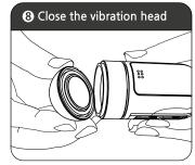
After winding up the cable, reattach the vibration head to the winder.
