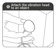
Tear off the protective film and then attach the vibration head to a hollow object such as empty boxes, plastic cups \*5).
