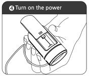
Insert 2 AAA batteries into the battery and then turn on the power switch, or use USB Power. \*3)
