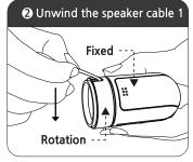
Hold the speaker body and then unwind the speaker cable clockwise or counter clockwise. \*2)
