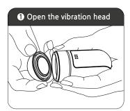
Hold the cable winder between your thumb and index finger, and open the vibration head with the other thumb. \*1)
