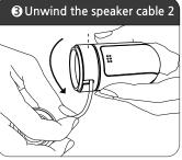
Hold the cable winder and then pull the vibration head.
